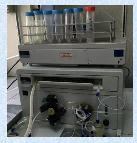
Flow injection mercury a system (FIMS)
