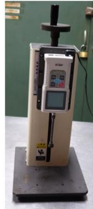
Aikoh digital force gauge Compression test (force and deformation)
